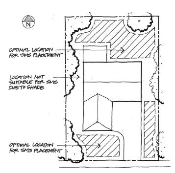
(Above left) Layout of irrigated areas showing optimal and unsuitable locations for sensor placement.
